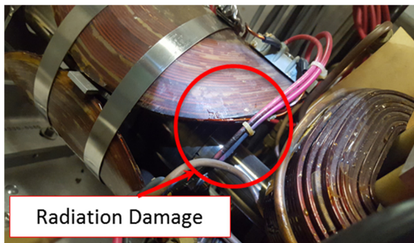
Figure 4: Showing effects of field emission induced radiation.
