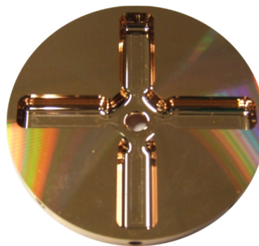
Figure 1: One cell of a CLIC high-power test accelerating structure. The part is made from OFE copper using a diamond tool and has micron-level tolerances. The four waveguides provide higher-order-mode damping (although no terminating loads are present here) and the outer cell wall is formed by four convex segments to minimize enhancement of surface current.
