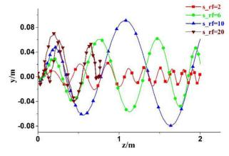
Figure 2: The projection of the motion of electron on the yz plane under different rf field strength S<sub>rf</sub>.
