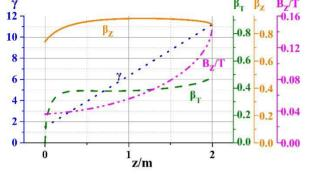
Figure 1: Dependence of initial guiding magnetic field B<sub>z</sub>, electron energy  $\gamma$ , transverse velocity  $\beta_T$  and axial velocity  $\beta_z$  on axial distance z in CARA (from z=0 to
