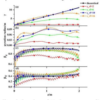
Figure 3: Dependence of (a) electron energy  $\gamma$ , (b) gyration radius  $\rho$ , (c) axial velocity  $\beta_z$  and (d) transverse velocity  $\beta_T$  on axial distance z at different  $S_{rf}$  value in CARA for a tapered axial magnetic field shown in Fig. 1.
