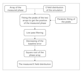
Figure 4: Flowchart of the data processing.
