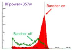
Figure 4: Measured bunch efficiency.
