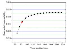
Figure 6: Frequency range of the DTL2 as a function of tuner position.
