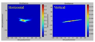
Figure 8: Measured transverse emittances at DTL1 exit.
