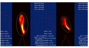
Figure 2: Measured transverse emittances after analysing dipole magnet.
