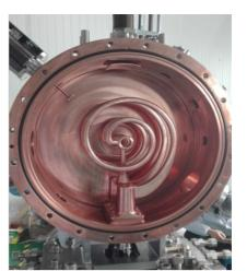
Figure 3: Spiral re-buncher cavity.
