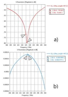
Figure 7: a) Reflected power  $(S_{11})$  b) Transmitted power  $(S_{21})$  of the power coupler.
