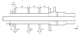
Figure 8: Scheme of a prototype power coupler for thermal analyses.
