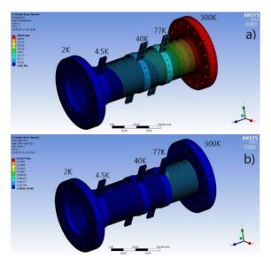
Figure 9: a) Temperature distribution and b) Heat flux result of static thermal load.
