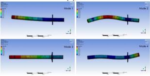
Figure 11: Four resonance modes of antenna.
