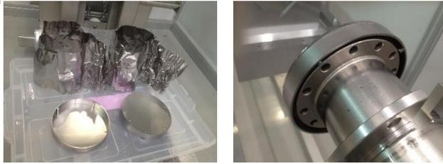
Figure 3: (left) Nb caps and foils to cover flanges. (right) Cavity flange covered with Nb cap.
