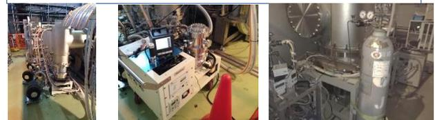
Figure 2: (top) Diagram for N-injection system. (left-bottom) TMPs and scroll pumps. (center-bottom) Portable pumping unit. (right-bottom) N-injection line.
