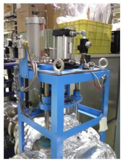
Figure 9: Old Safety Shutter: Oil-Hydraulic Cylinder.
