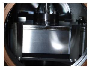
Figure 11: New Safety Shutter: 250-mm Thick Tungsten Block.
