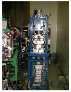
Figure 8: Old Safety Shutter: 400-mm Thick Stainless Steel Block.
