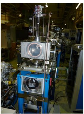
Figure 10: New Safety Shutter: 250-mm Thick Tungsten Block with Pneumatic Cylinder.
