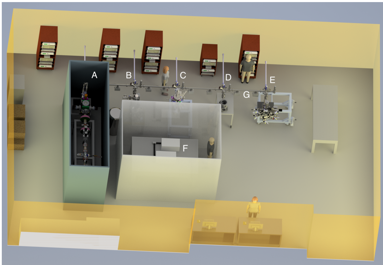
Figure 1: 3-D model of the ASU Photocathode lab (currently under development). The letter labels correspond to the following (A) 200 kV DC Electron Gun with diagnostics/UED beamline; (B) Electron Energy Analyzer; (C) Alkali-Antimonide Growth Chamber; (D) Surface Diagnostic Chamber; (E) Single-Crystal Growth Chamber; (F) Tunable wavelength laser (G) UHV transfer line.
