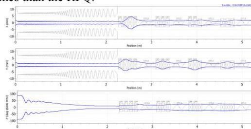
Figure 4: Rms-envelopes of the beam in the linac.
