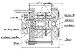
Figure 1: Magnetron proton source.
