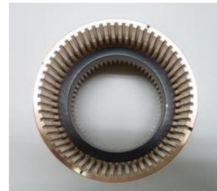
Figure 6: A copper cylinder brazed with an AlN cylinder.
