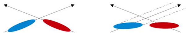
Figure 2: Schematic of the bunch crossings at the IP with and without crab cavities.
