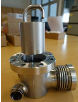
Figure 8: Bottom: DQW HOM coupler in bulk Nb with its stainless steel jacket for active cooling (courtesy CERN EN-MME).
