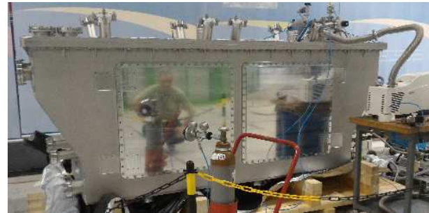
Figure 9: Top: The two-cavity cryomodule hosting the crab cavities (left) and the top loading assembly sequence (right). Bottom: Vacuum vessel under vacuum testing (courtesy CERN EN-MME).
