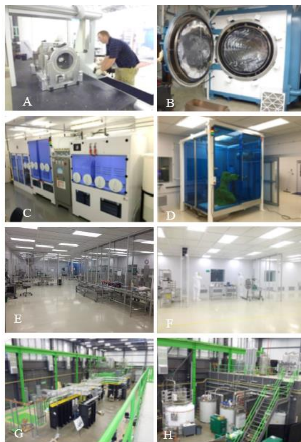
Figure 8: Many cavity production equipment in the SRF Highbay. A: CMM machine to dimensional inspection, B: Vacuum furnace for hydrogen degassing, C: BCP facility, D: Robotic HPR system, E: Large cleanroom, F: Class 10 cavity assembly clean-room, G: Cavity vertical test system, H: Dedicated 900W liquid helium refrigerator and 5000L storage Dewar.
