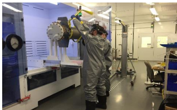
Figure 9: View of BCP processing in the chemi room in SRF highbay.
