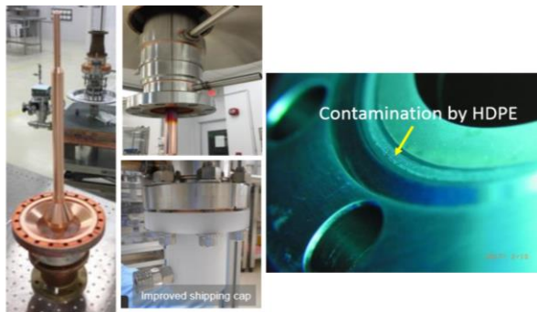
Figure 14: MPF coupler on left, shipping cap in middle, and contamination on the ICF flange by HDPE on right.
