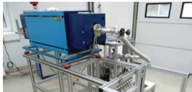
Figure 16: Image of the small sample furnace. The furnace has a ceramic tube with a diameter of 80 mm. A Residual Gas Analyzer and a mass-flow controller for nitrogen inlet is installed. The maximum achievable, stable temperature is 1350°C. The pump system is completely oil free and achieves  $p < 2 \times 10^{-7}$  mbar. The furnace has been setup for dedicated nitrogen-infusion studies on samples.
