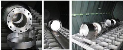
Figure 14: Illustrated cavity installation for the nitrogen infusion of 1DE7. To mimic the line of sight protection a dummy cavity (instead of the niobium box) is used shown on the left picture. The sample “outside” is placed on a ceramic plate to make sure to have a clean underground for the sample.
