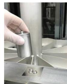
Figure 2: Coverage of cavity witness samples beneath a HOM coupler to mimic LOS protection of the caps.
