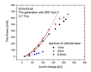
Figure 4: Measured THz power vs. bunch charge.
