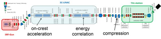
Figure 1: The ELBE beamline layout for the THz radiation production with the SRF gun and Linac.
