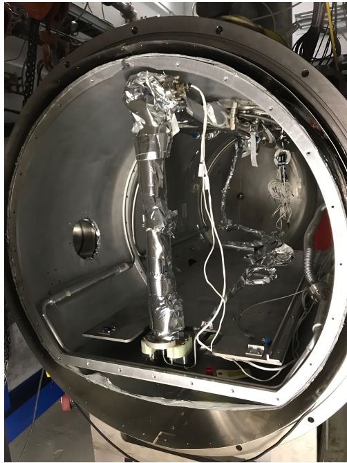
Figure 9: Inside of the upgraded STC cryostat: prepared for commissioning 0-cavity cool down.
