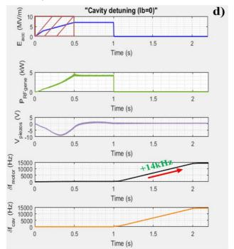
Figure 7: Evolution versus time for the faulty cavity without beam.
