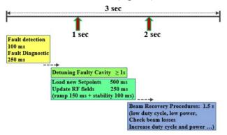
Figure 3: Fault tolerance tests (specification for MYRRHA  $\leq 3s$ ).
