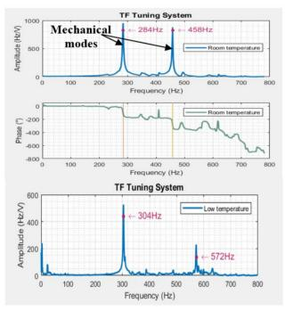
Figure 8: TF of the Tuning System at room T (up, MYRRHA single Spoke cavity « Virginia ») and low T, T<sub>He</sub>=2K (down, cavity « Amelia »): detuning on the RF frequency of the cavity according to the low frequency excitation of one of the piezoelectric actuators.
