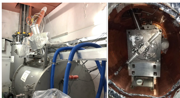
Figure 7: The photos of the dressed cavity installed in the modified cryomodule.
