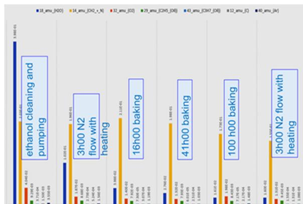
Figure 6: RGA histograms of the different species with reference to nitrogen during the different cleaning steps of the N<sub>2</sub>-line.
