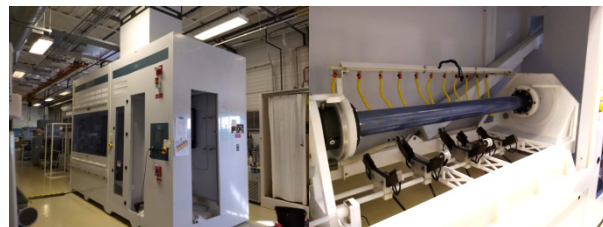
Figure 7: Large EP tool at FNAL CPL (left) and a dummy tube installed for flow test on EP bed (right).
