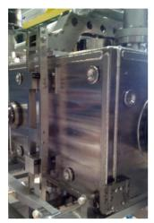
Figure 4: Tuning frame and flexural guides on the DQW helium tank.
