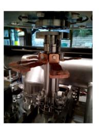
Figure 6: The concentric tuning tubes with thermalisation.
