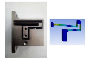
Figure 5: Flexure guide design.
