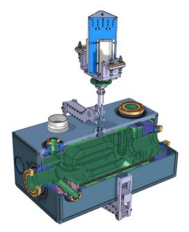
Figure 1: Cut-away view of the RFD tuner.
