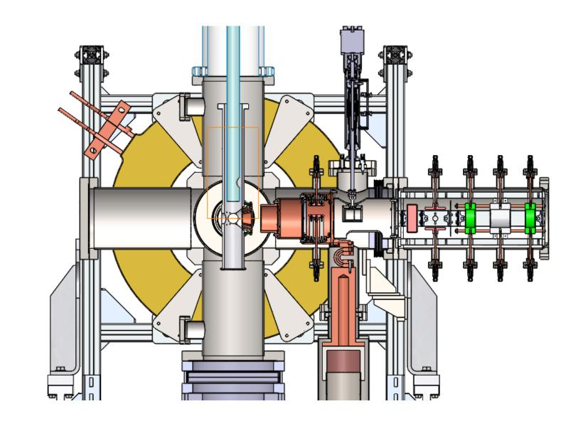
Fig.6. The new 200 mT Helmholtz coil magnet and the support stands/bracket design
