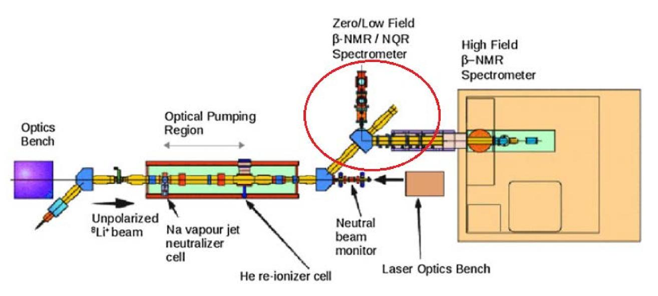
Fig.2. Current existing  $\beta$ -NMR beamline. Circled in red is the location of the  $\beta$ -SRF upgrade [G. Morris, 2014]
