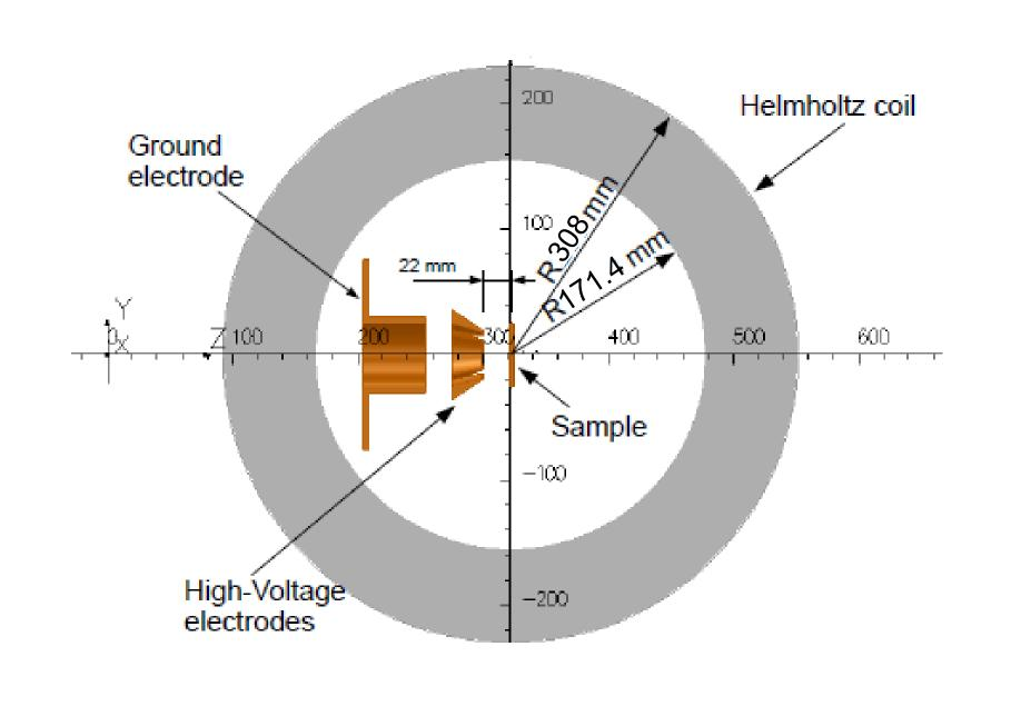
Fig.4. The modified optics and a new fourelectrode segmented decelerator used for compensation of the higher magnetic field and deceleration of beam (modified from [S. Saminathan, 2015])
