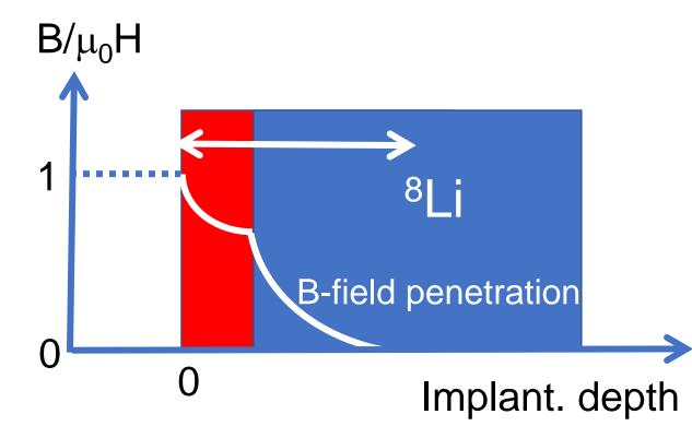
Fig.1. Measurements of penetrating field in the Meissner state with radioactive <sup>8</sup>Li
