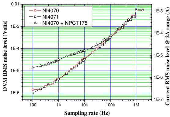
Figure 2: Noise test result of DVM and NPCT.
