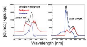
Figure 3: First BCD measurements with 230-µm thick organic DAST crystal compared with EO signals with a 1-mm inorganic ZnTe crystal. The both of the crystals were set 2.0 mm from the electron beam axis.
