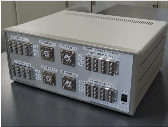
Figure 6: Signal switching box (front view).
