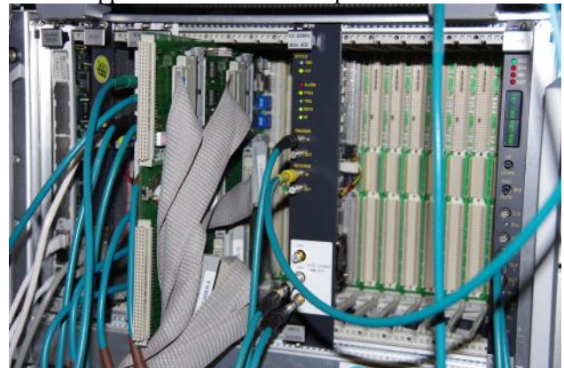
Figure 4: 18K10 in the VME subrack. VME extension left to the 18K10 is used to monitor the VME bus timing using logic analyser.
