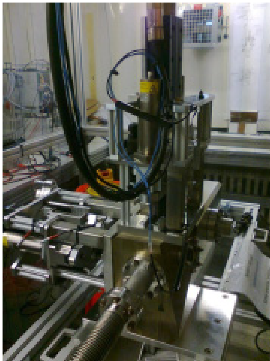
Figure 5: XFEL wire scanners' test setup
