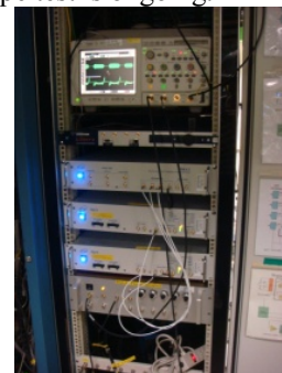
Figure 4: Prototype electronics for bunch-by-bunch feedbacks.
