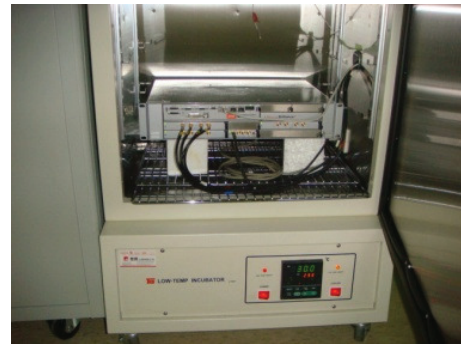
Figure 11: Libera Brilliance+ platform put inside an incubator which provide precision temperature control in the range between 0~60 °C. Measurement is performed around 30°C.
