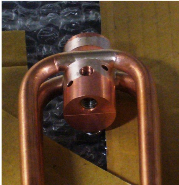
Figure 2: Copper mirror mount.
