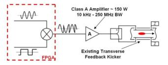
Figure 6: Bunch cleaning system layout.
