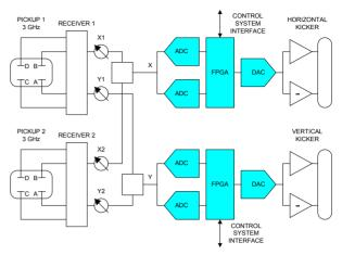
Figure 1: ALS Transverse Feedback Electronics.
