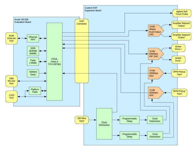
Figure 2: ALS Transverse Feedback Hardware Block Diagram.
