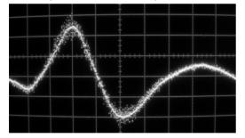
Figure 3: Close-up at the 100 KHz 20% amplitudemodulated impulse (notice the fuzzy samples around the tip of the impulse due to very small amplitude modulation, scale 10mV/div, time scale 100 ps/div)
