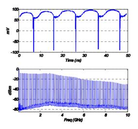
Figure 1: The impulse train generated using the 100 MHz HP-33002 snap diode in time domain (above, with 30 dB attenuation) and spectrum content (bottom, showing the 100 MHz comb)
