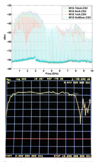
Figure 4: Lab measurement results of Marki M8-0412. The top figure is measured on the spectrum analyzer by driving M1J with a small modulation and a DC current of 1 mA (red), 5 mA (green), and 10 mA (blue). The bottom figure is from the network analyzer, frequency spanning from 50 MHz to 10.05 GHz, 10 dB/div.
