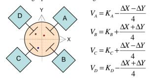
Figure 10: Button-style Beam-Position Monitor and the relationship between the Four-button voltages and the Beam Position
