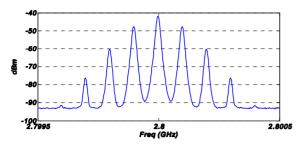
Figure 2: Simulated Synchrotron oscillation (DC voltage with 100 KHz modulation)
