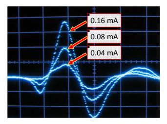
Figure 7: Linear Response of the Modulator. Snapshot of the impulse when the mixer is operating at DC control currents of 0.04 mA, 0.08 mA, and 0.16 mA. Time scale 10 mV/div, time scale 100 ps/div.
