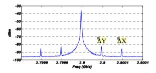
Figure 11: Spectral content of the one bunch signal with oscillations on  $\Delta X$  and  $\Delta Y$ .
