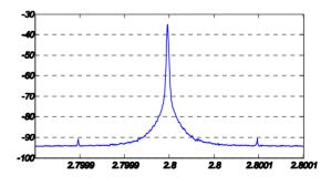
Figure 8: 60 dB carrier-to-sideband ratio, centered at 2.865 GHz, sidebands 100 KHz apart
