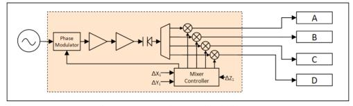
Figure 9: One Bunch system block diagram.
