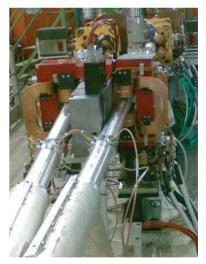
Figure 4: One of the gamma monitor installed between the two last correctors and the final permanent quadrupoles of DAFNE IR.
