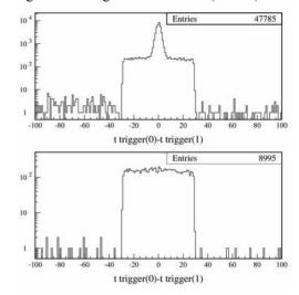
Figure 9: (top) Bhabha time of arrivals in the opposite modules as selected by the T1FREE hardware trigger. (bottom) background time of arrivals when the beams are not colliding (180 degree longitudinal separation)
