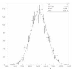
Figure 7: energy resolution of  $14\%\sqrt{E(GeV)}$  obtained at the test beam with 470 MeV electron impinging the center of one of the 20 sectors.
