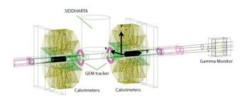
Figure 6: GEANT simulated setup
