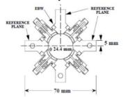
Figure 3: ATF damping ring button BPM.
