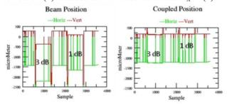
Figure 12: Uncorrected (left) and corrected (right) beam position measurements using the CAL system.
