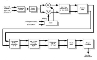
Figure 7: Digital signal processing in the Graychip DDC.
