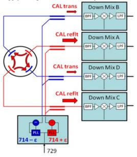
Figure 6: BPM calibration system.
