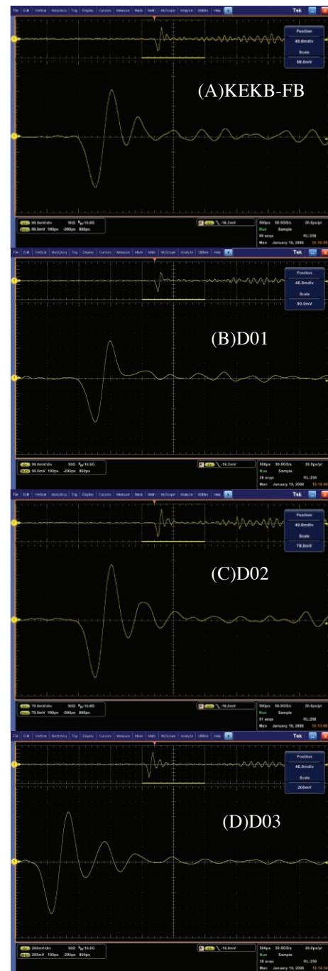
Fig. 19. Beam response of BPMs from linac beam.
