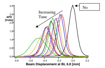
Fig. 11: Beam profile at different tunes for pass #5.
