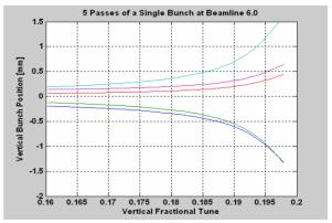
Fig. 8L Separation of the five passes vs. tune.
