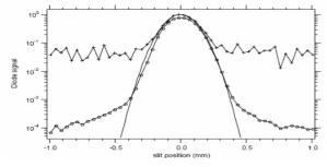
Fig. 3: Measured horizontal profile at BL 5.3.1 at 5 keV. The crosses and circles represent two amplifier gains and the line without symbols shows a Gaussian fit (Data
