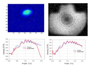
Figure 4: Unfocused beam (no-waist, solenoid only). Top – beam spot distribution (black circle is an interferometer aperture with diameter 15mm); top right – image of the angular distribution of intensity; bottom left and right are the horizontal-x and vertical-y scans of angular distribution
