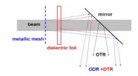
Figure 1: Mesh-dielectric foil interferometer.
