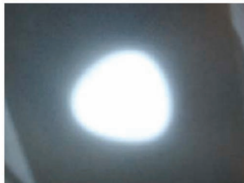
Figure 1: Beam imaging of a \text{He}^+ beam with the tantalum sheet, left, shows triangular beam structure 80 cm after extraction.
