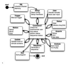
Figure 3. The State-machine structure.
