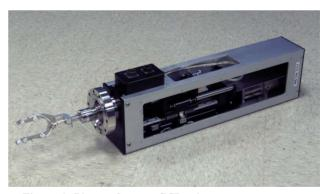
Figure 1. Photo of a new CCL wire-scanner actuator.
