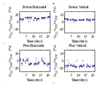
Figure 6 shows the percentage differences between the Synclite and Flying Wire emittances for a handful of beam stores.
