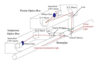
Figure 5. Synchrotron Light Monitor.
