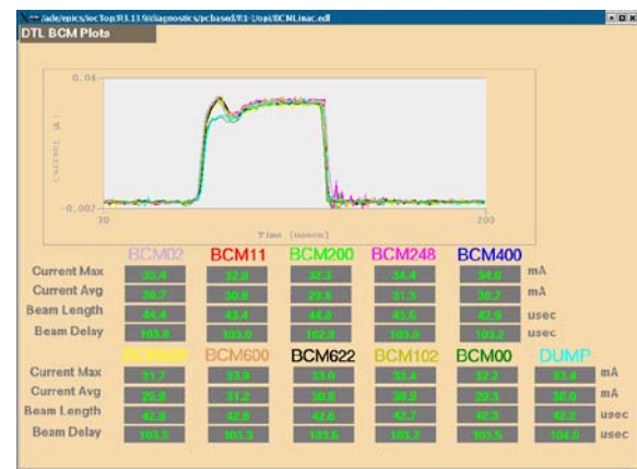
Figure 1. A beam pulse transmission from the injector to the linac beam dump measured by linac Beam Current Monitors.
