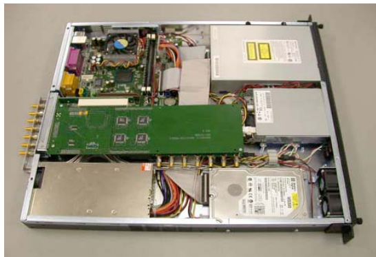
Figure 2. The BPM PCI card inside the PC chassis.
