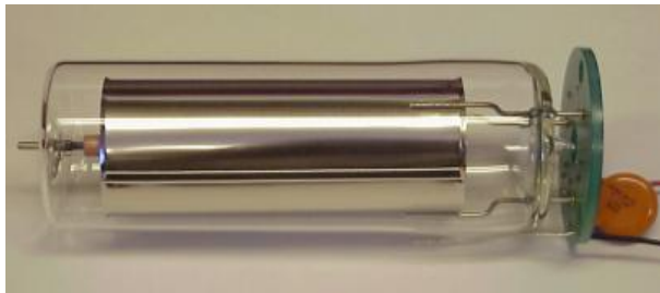
Figure 9: SNS ionization chamber. Contents = 113 cm 3 of argon; HV= -1000V; sensitivity 70 nC/rad.
