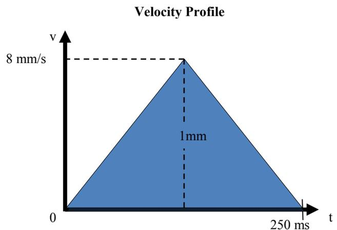
Figure 1: Velocity profile for the wire scanner.
