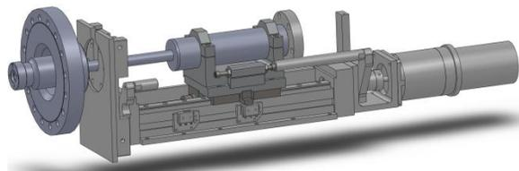
Figure 2: ORNL SNS wire scanner design.
