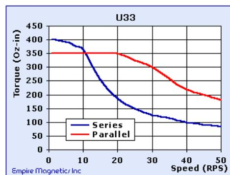
Figure 4: EMI U33 stepper motor speed vs. torque curves.
