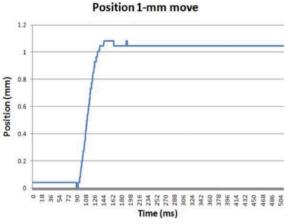
Figure 4: Plot of position of 1-mm move.
