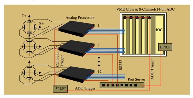
Figure 1: The ATF2 BPM processing system block diagram.
