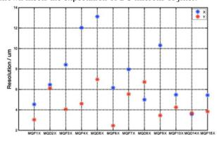
Figure 3: Estimate of the resolution for 12 BPMs.
