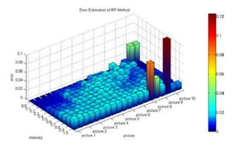
Figure 4: Error Estimation of the IRF-Method on nine numerical and one measured picture. For every picture the upper and the lower isolumens were computed and estimated with  $\chi$ .
