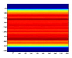
Figure 7: Picture 8 shows a strongly defocused beam that was computed numerically. Dark lines in the middle are numerical artifacts, which significantly could disturb the proper determination of isolumens, because unambiguousness gets lost.
