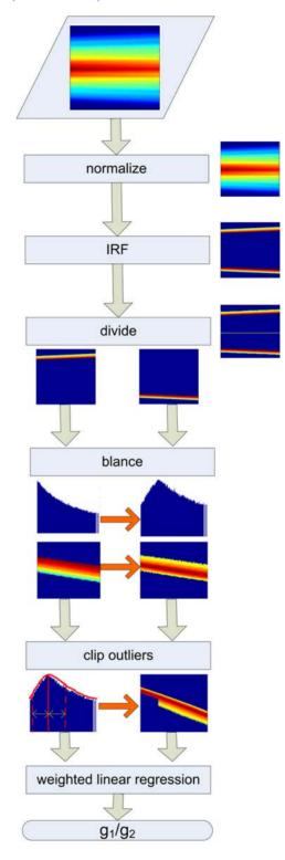
Figure 2: The IRF-method determines isolumens sensitive to information.
