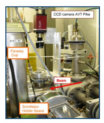
Figure 3: Ion Beam-Material Irradiation Test Setup at the Max- Planck Institute in Heidelberg.
