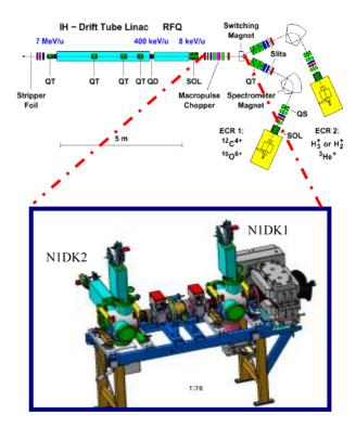
Figure 1: The Low Energy Beam Transport at HIT and the position of the Pepper-Pot Scintillator Screen device within the LEBT (Low Energy Beam Transfer).
