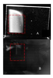
Figure 4 A-B: The degradation of YAG:Ce after a total irradiation of 2000 ms (which is equivalent to 1.4 \*10^14 particle per pulse) can be seen in picture B.
