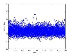
Figure 6: The beam lifetime measurements after the unstable ones are discarded.
